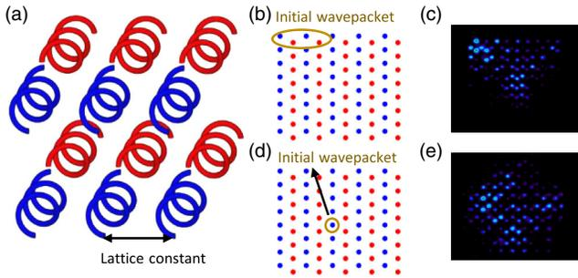
FIG. 3. (a) Helical waveguide array in a diagonal lattice with shifted helicity (as in Ref. [33]). (b),(d) location of input beam when the edge states are excited (b) and when the edge states are not excited (d). (c),(e) Example of experimental output intensity images, when the input wave packet is on the upper edge (c), and when the input is in the middle of the lattice (e).
